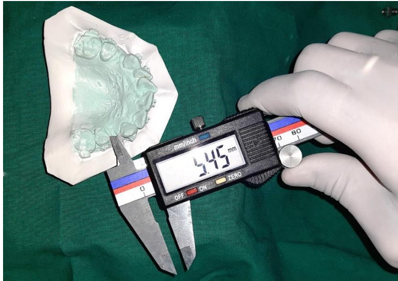
Figure 3. Measurement of tooth movement with digital vernier calliper
